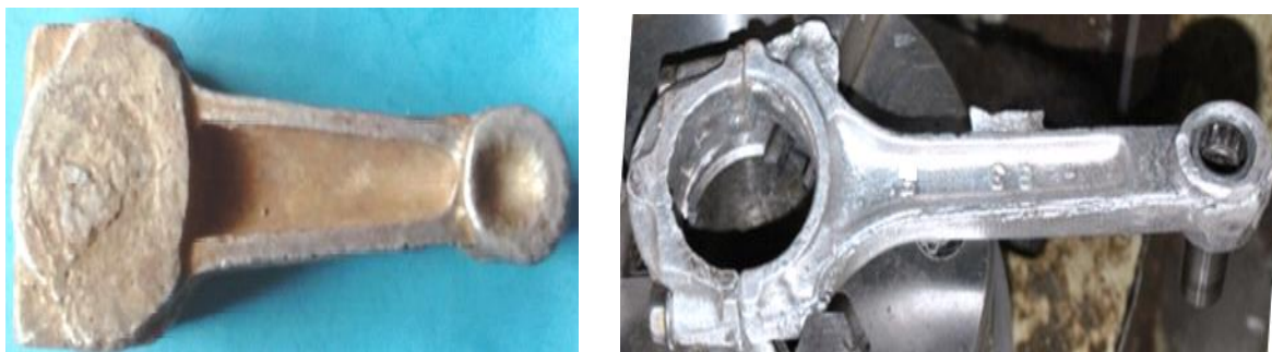
(a) (b) Fig. 5(a) and (b) Image of the produced connecting rod. (a) before machining and (b) after machining
