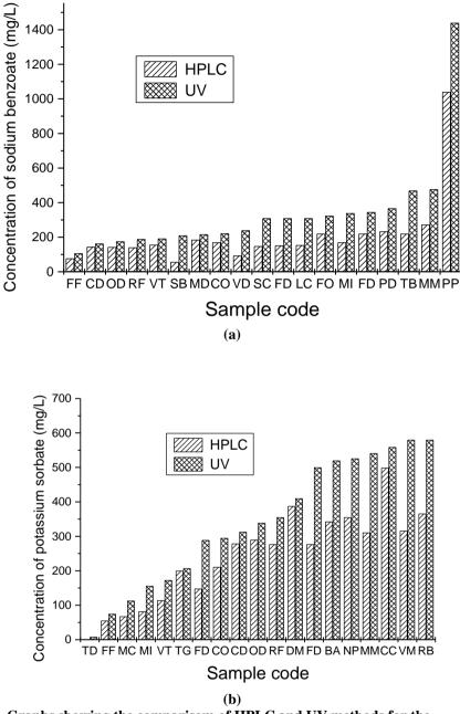
Fig. 2: Graphs showing the comparisom of HPLC and UV methods for the determination of sodium benzoate (a) and potassium sorbate (b)
