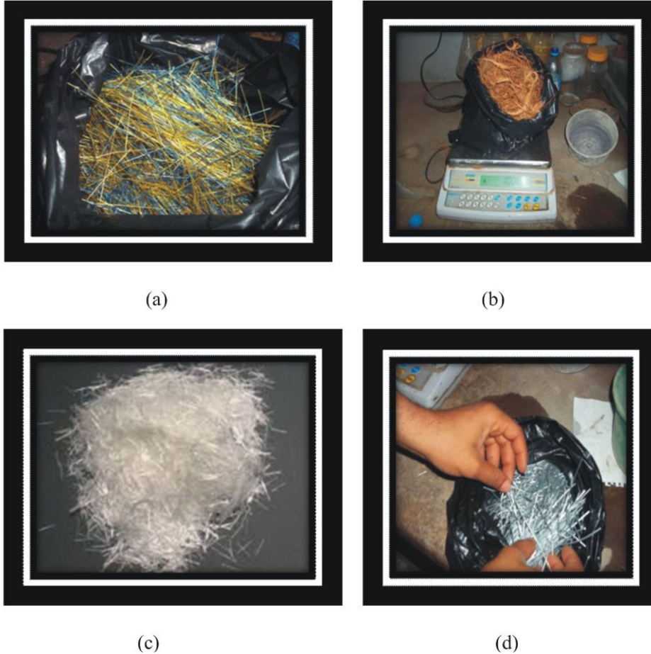
Fig. 1: Fibres used as reinforcement: (a) polymeric fibre, (b) coconut fibre, (c) glass fibre, and (d) steel fibre
