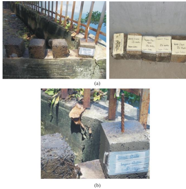
Fig. 4: Concrete cubes after immersion in natural Corrosive environment: (a) sets of corroded cubes and (b) typical corroded rebar concrete cube with scales
