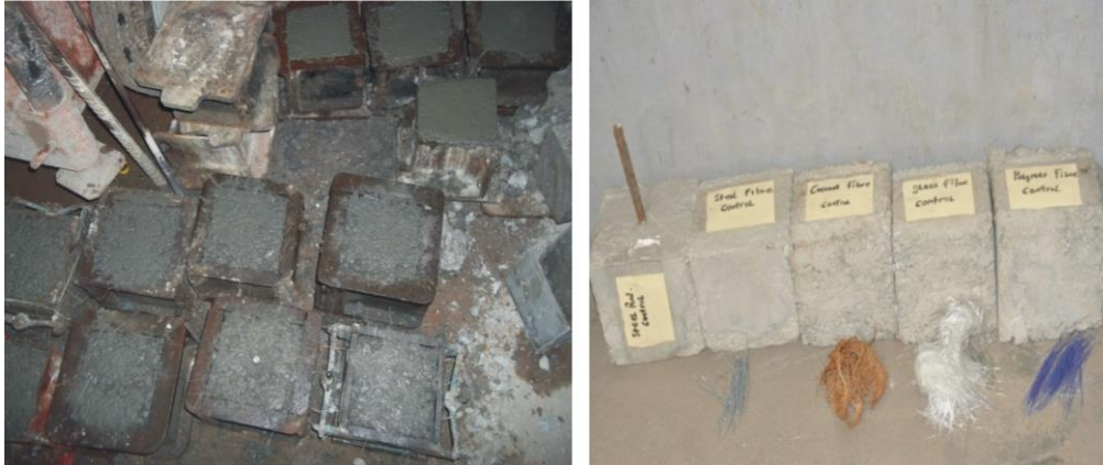
Fig. 2: Image acquisitions of cast rebar and FRC cubes after curing
