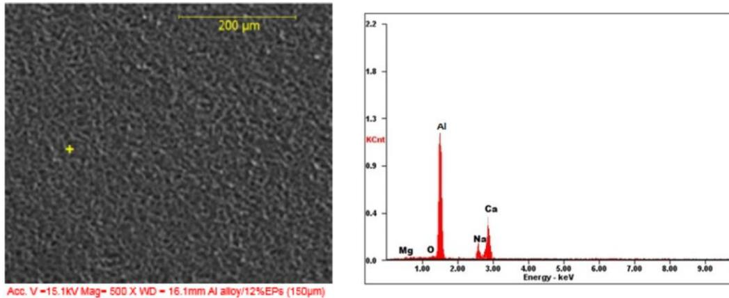
Fig 6: SEM/EDX of Al alloy/12% ESp (150µm) composites
