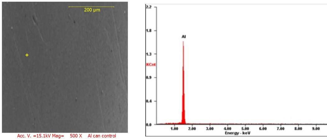
**Fig 2: SEM/EDX of Al alloy (control)**
