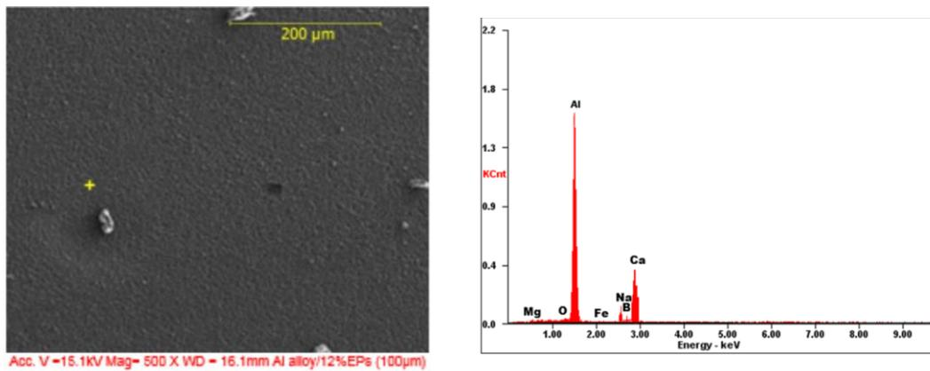
Fig 5: SEM/EDX of Al alloy/12% ES (100µm) composites
