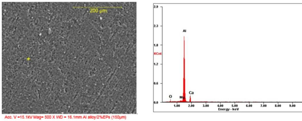
Fig 4: SEM/EDX of Al alloy/2% ES (150µm) composites
