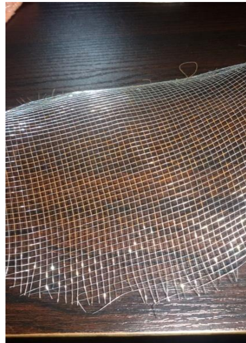
Plate 2b: 0.3cm Smoke Filter Used in EFK
