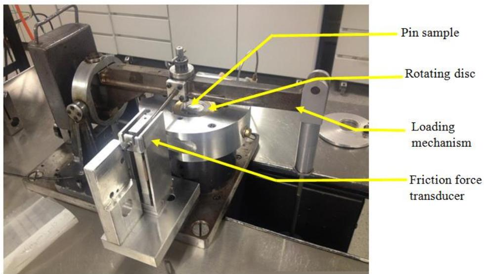
**Plate 1: Denison T62 HS pin-on-disc wear-testing machine (Leeds, UK)**
