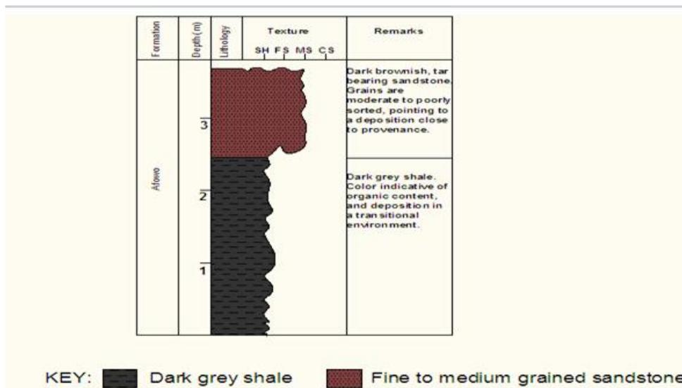
Fig 6: Lithologic section of Area J4 sequence
