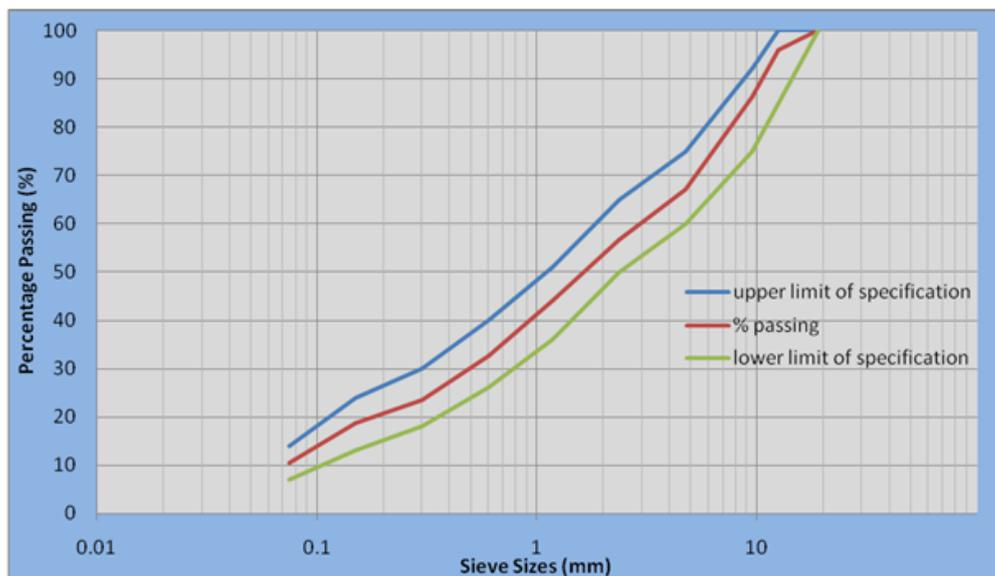
Fig 9: Gradation results for all upgraded tar sand samples
