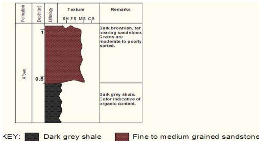
Fig 3: Lithologic section of Imeri sequence
