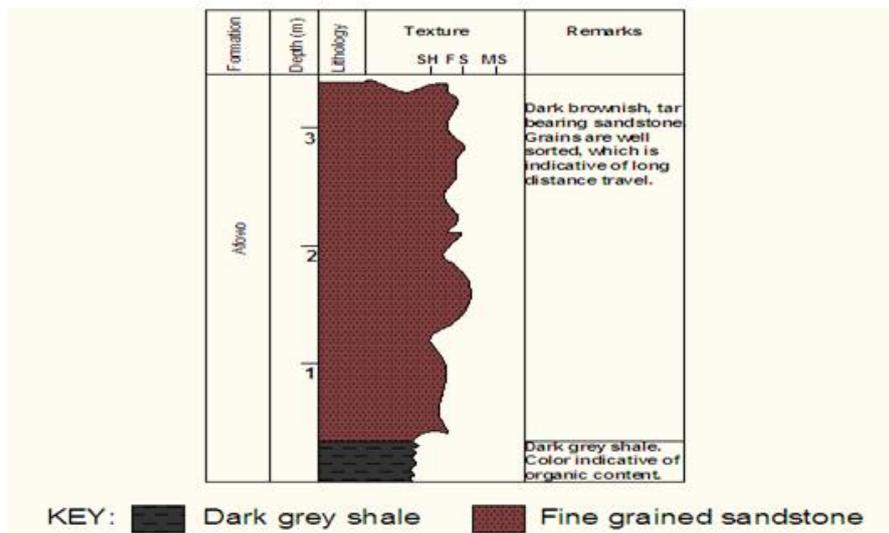
Fig 5: Lithologic section of Loda sequence
