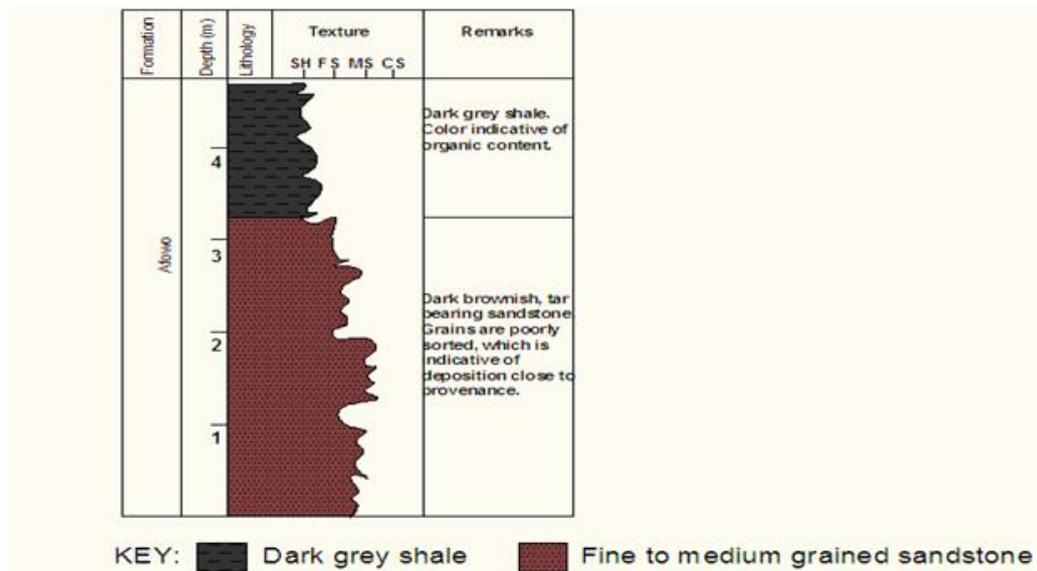
Fig 7: Lithologic section of Idobilayo sequence
