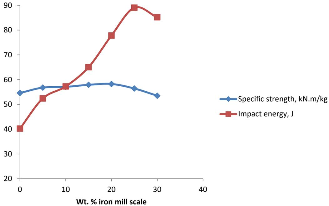
Fig. 1: CMC specific strength/Impact energy variations with iron mill scale addition
