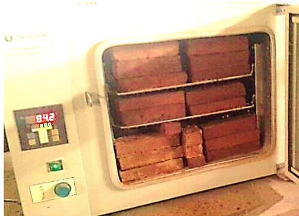
**Figure 1: Samples of alkali activated lateritic mortar prism stockpiled in the oven for curing**
